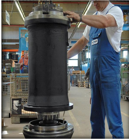
Assembling the Large Pump.
